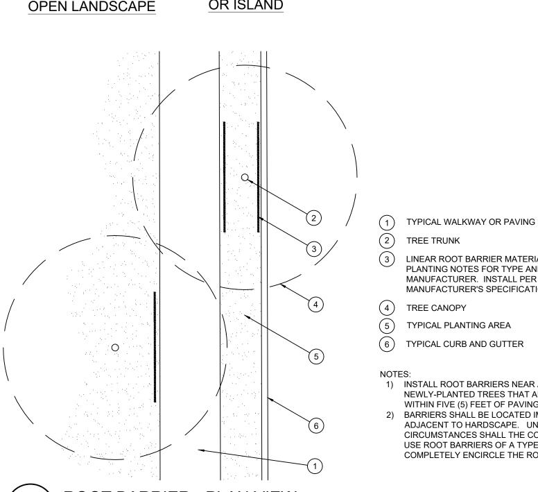
LINEAR ROOT BARRIER MATERIAL. SEE PLANTING NOTES FOR TYPE AND MANUFACTURER. INSTALL PER MANUFACTURER'S SPECIFICATIONS. TREE CANOPY (5) TYPICAL PLANTING AREA
